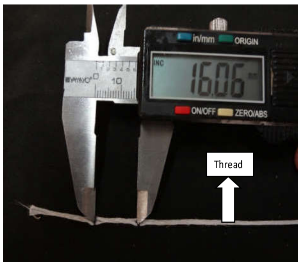
Fig. 3: Measurement of internal diameter of femoral artery: Distance between the two points on the thread is measured by digital vernier caliper
